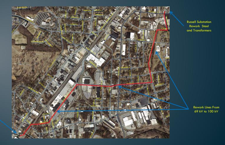
Burton Substation Rework Steel and 69kV/100kV Transformer
