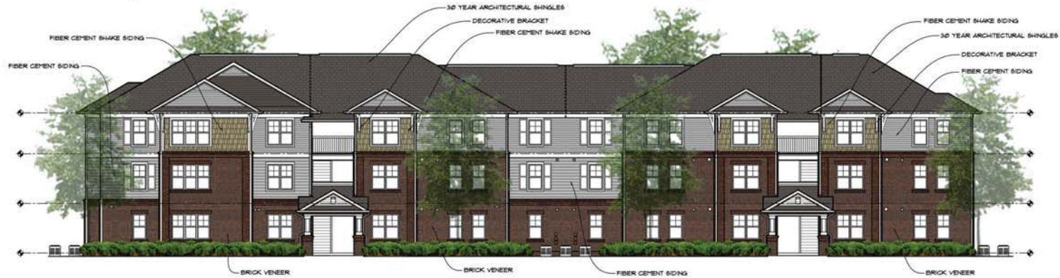
1 BUILDING 100 & 200 - FRONT ELEVATIONS 1/8" = 1'-0"
